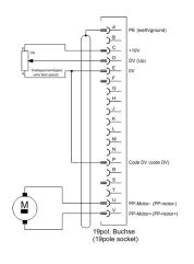
with potentiometer for wire feed speed
