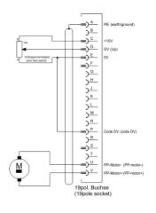
with potentiometer for wire feed speed
