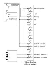
with potentiometers for wire feed speed and arc length correction
