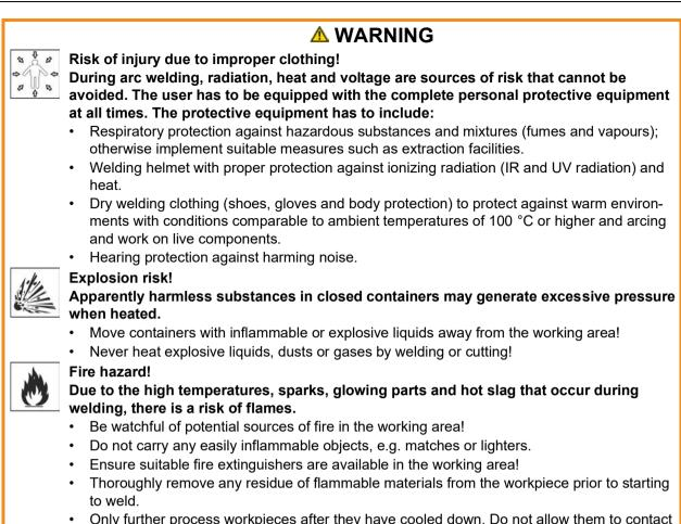
• Only further process workpieces after they have cooled down. Do not allow them to contact any flammable materials!
