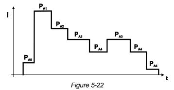
Example 3: Aluminium welding of different sheet metal thicknesses (non-latched or latched special)
