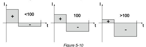
The AC amplitude balance can be set in the Expert menu (TIG) using parameter  $\frac{RbR}{}$  > see 5.2.11 chapter.
